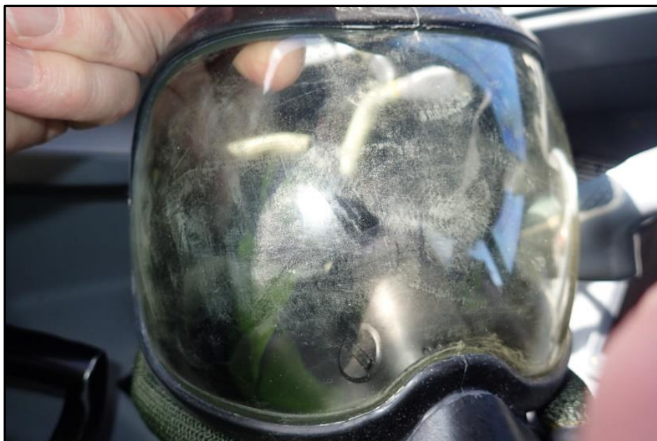
Photo No. 2: Co-Pilot's Smoke Goggles showing obscuring layer on inner surface
